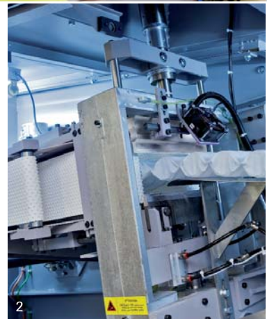
1 Ultrasonic cutting of precision fabric for screen-printing.
