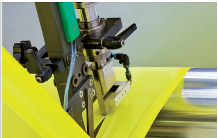
2 Textiles ultrasonic welding of pocket springs.
